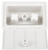
RV Exterior Spray Box Spray Box and Faucet with Quick Connector, use with DF-SA183 or DF-SA187. Mount Cutout: 7.375"W x 4.125"W Outside Dim: 8.875"W x 5.625"H x 4"D
