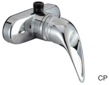
Single Lever RV Shower Faucet Non-Metallic, Vacuum Breaker Hose Connection, Ceramic Disk MFG# DF-SA150-CP Finish Chrome (CP) DF-SA150-ORB Oil Rub. Bronze (ORB) DF-SA150-SN Satin Nickel (SN) DF-SA150-WT White (WT)
