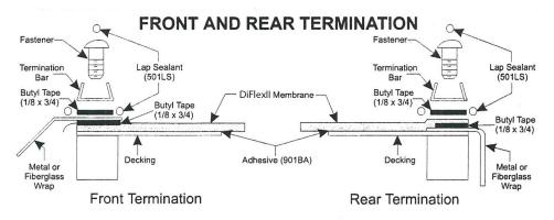
NOTE: Butyl tape should also be used under the TPO membrane where it comes in contact with the unit body at the front, rear, and side terminations. See all termination drawings for correct butyl placement.
