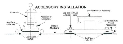
Caulk all screw heads, front and rear termination bar and all accessories. Note: Only Butyl Tape can be used with DiFlex II<sup>™</sup> membrane to assure proper seal.
