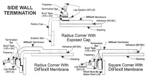
8. Apply butyl tape (BT-1834) to the termination molding. On the front of the vehicle, the front cap should lay on top of the membrane. Using a screw-type fastener, install the termination moldings – making sure there is sufficient roof structure. On the rear of the vehicle, the membrane should lay on top of the rear cap.
