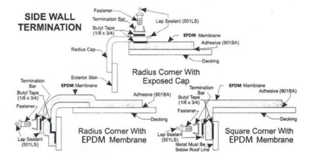
8. Apply butyl tape (BT-1834) to the termination molding. On the front, the front cap should lay on top of the membrane.
