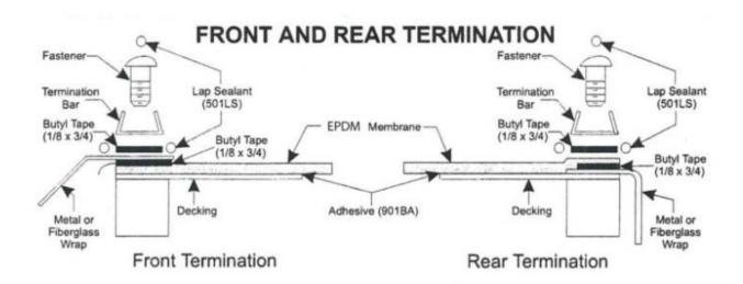
**NOTE:** Butyl tape should also be used under the EPDM membrane where it comes in contact with the unit body at the front, rear, and side terminations. See all termination drawings for correct butyl placement.
