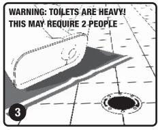
Remove toilet – you may need to gently rock the toilet to break the seal. Lay down large towel or old rug and relocate toilet onto the rug. CAREFULLY lay the toilet on its side or tilt toilet and wipe off old, waxy residue from underside of toilet base with paper towels.
