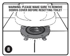
Line up bolts through the holes in base and reset the toilet. Tighten nuts to secure toilet to the HydroSeat. Do not overtighten. Reconnect water supply line (we recommend replacing old, stiff supply line, with a new flexible supply line) Turn on water and check supply line for leaks. Allow toilet to fill. Flush to check for leaks.
