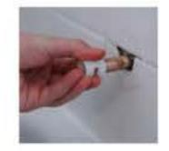
Slide the Adapter onto the Stub Out Nipple with the threads toward the wall. Lubricate the Stub Out Nipple tubing about 1" with Silicone Grease.
