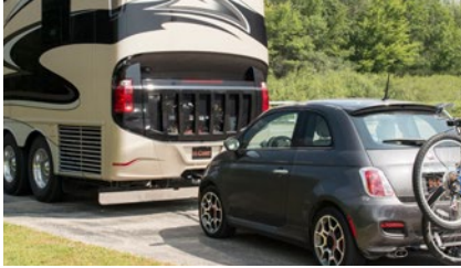
Connects a towed vehicle to an RV using a standard 4-way flat trailer plug
