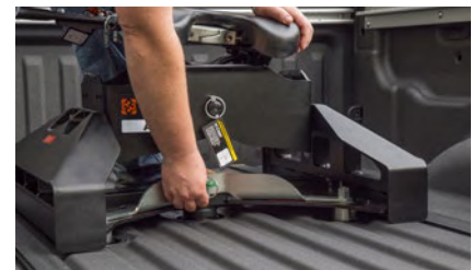
Step 3 - Secure levers with attached safety pins and you're ready to hitch up your trailer
