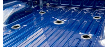
Installation of these products requires an OEM truck bed puck system (see above example, Ram puck system)
