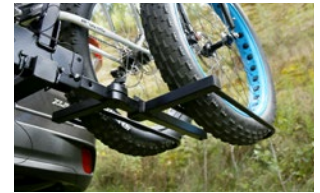
18091 fat tire cradles replace existing cradles on CURT racks
