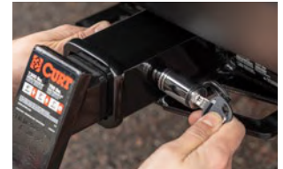
Easy-to-operate, 1/4-turn lock activation
