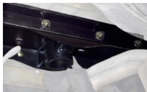
Step 2 - Bolt the install brackets and hitch to the vehicle frame
