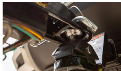
Fastens securely with included 1/2" diameter pin and clip (also accepts a 1/2" hitch lock)
