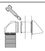
When connecting to a wall pipe, cut a 1" long slit in tailpipe. Position a clamp so it covers the slit in the vent tailpipe. Insert crimped fitting into tailpipe. Tighten clamp
