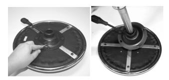
Use an allen wrench to attach the Seat Plate to the underside of the Seat with the provided Screws. Insert the Support Cylinder into the center of the Seat Plate
