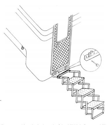
Note: be sure there are no electrical wires, water lines or anything else in the path of the drill bit before you drill.
