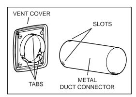
3. Connect METAL DUCT CONNECTOR together. Snap SLOTS in DUCT into TABS on VENT COVER.
