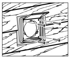
Secure vent cover to wall with 4 SCREWS (included). Caulk around vent cover with a quality caulking compound.
