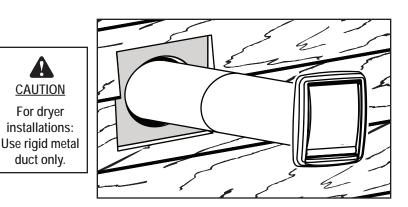
5. Insert duct through hole in wall and fasten duct to metal duct connector. Use duct tape on all connections to make them secure and air-tight.
