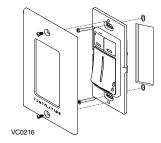
Perform the electrical connection to the connector of the unit, as shown below. For more details, refer to the installation manual of the ventilation unit.
