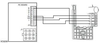
**8** Plug the ventilation unit and test the wall control.
