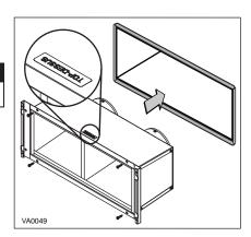
Assemble the grille to the metal tandem hood box using both  $n^{\circ}$ . 8 x  $3/8^{\circ}$  screws previously removed PLUS 2 OTHER  $N^{\circ}$ . 8 x 3/8" SCREWS FROM PARTS BAG. SEAL THE OUTLINE WITH CAULKING.
