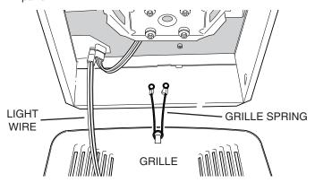
Remove fan GRILLE by squeezing two GRILLE SPRINGS and sliding them out of their mounting slots on each side of the fan housing. Disconnect LIGHT WIRE from fan (if fan is equipped with a light). Set grille assembly aside for now.
