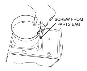
14. Install 6" DUCT CONNECTOR (S) to fan housing and secure with screw supplied in fan parts bag.
