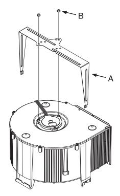
Assemble SUPPORT BRACKET (A) (supplied with radiation damper) to fan blower as shown. Secure the bracket to motor studs with (2) #8-32 HEX NUTS (B) supplied in radiation damper parts bag.
