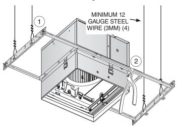
16. If the fan is directly mounted to adjacent ceiling structure, use #8 (M4) SHEET METAL SCREWS OR ¼"DIAMETER BOLTS WITH NUTS to fasten SLIDING HANGER BARS. Sliding hanger bars are provided to allow for accurate positioning of fan between ceiling members.
