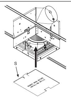
18. Install **MASK (S)** supplied with the fan to protect damper and fan from drywall spray, construction dust, etc.
