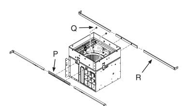
13. Attach MOUNTING CHANNELS (P) to housing using SCREWS (Q) supplied in fan parts bag.
