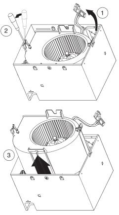
1. Remove blower and all packing material from fan housing.
