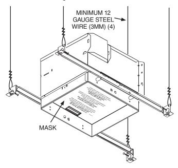
11. If the fan is directly mounted to adjacent ceiling structure, use #8 (M4) SHEET METAL SCREWS OR ¼" DIAMETER BOLTS WITH NUTS to fasten SLIDING HANGER BARS. Sliding hanger bars are provided to allow for accurate positioning of fan between ceiling members.
