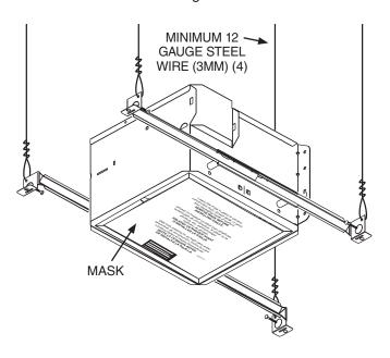
4. If the fan is directly mounted to adjacent ceiling structure, use #8 (M4) SHEET METAL SCREWS OR 1/4" DIAMETER BOLTS WITH NUTS to fasten SLIDING HANGER BARS. Sliding hanger bars are provided to allow for accurate positioning of fan between ceiling members.
