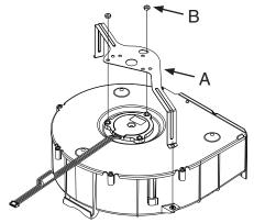
Re-install blower into fan housing.
