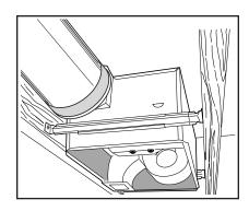
ductwork connections to make them secure and air tight.
