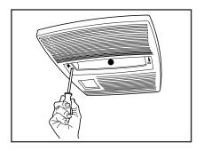
To avoid damage to the grille: DO NOT OVERTIGHTEN SCREWS. Tighten screws only until grille is snug against ceiling material.
