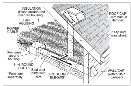
The ducting from this fan to the outside of the building has a strong effect on the air flow, noise and energy use of the fan. Use the shortest, straightest duct routing possible for best performance, and avoid installing the fan with smaller ducts than recommended. Insulation around the ducts can reduce energy loss and inhibit mold growth. Fans installed with existing ducts may not achieve their rated airflow.
