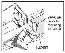
material, position bottom of each mounting flange flush with the bottom of joist. The housing mounts with four (4) screws or nails. Screw or nail housing to joist through lowest holes in each mounting flange, then through highest holes. NOTE: Mounting to I-JOIST (shown) requires use of SPACERS (included) between the highest hole of each mounting flange and the I-joist.
