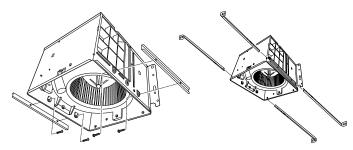
Sliding hanger bars are provided to allow for accurate positioning of housing anywhere between framing. They can be used on all types of framing (I-joist, standard joist, and truss construction) and span up to 24."
