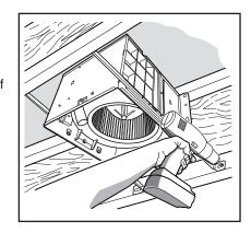
To ensure a noise-free mount: Secure hanging bars together with SCREWS and use a pliers to crimp mounting channels tightly around hanger bars.
