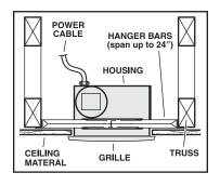
Housing mounted anywhere between <u>trusses</u> using <u>hanger bars</u>.
