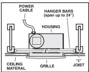
Housing mounted to joists.
