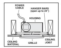
Housing mounted anywhere between <u>trusses</u> using <u>hanger</u> bars.
