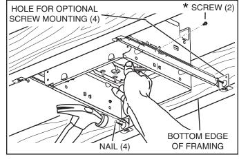
Extend HANGER BARS to the width of the framing.
