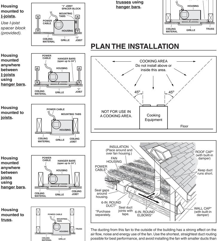
possible for best performance, and avoid installing the fan with smaller ducts than recommended. Insulation around the ducts can reduce energy loss and inhibit mold growth. Fans installed with existing ducts may not achieve their rated airflow.
