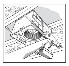
To ensure a noise-free mount: Secure hanging bars together with SCREWS and use a pliers to crimp mounting channels tightly around hanger bars.
