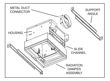
Assemble support angles and duct connector to ventilation fan housing:
