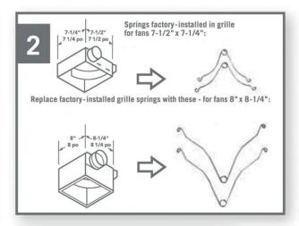
Attach new grille to fan with one grille spring (nearest to fan receptacle). Plug motor into pass-thru plug. Plug pass-thru plug into fan receptacle.
