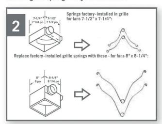
Attach new grille to fan with one grille spring (nearest to fan receptacle). Plug motor into pass-thru plug. Plug pass-thru plug into fan receptacle.
