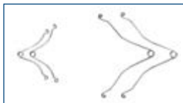
Choose grille springs matched to your fan model. Left: Factory-installed grille springs for fan models: 688, 671, 678 and 771. Right: Replace factory-installed grille springs with larger springs for fan models: 770, 676, 679 and 683.
