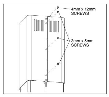
20. Carefully place the (2) upper flue sections on the hood
