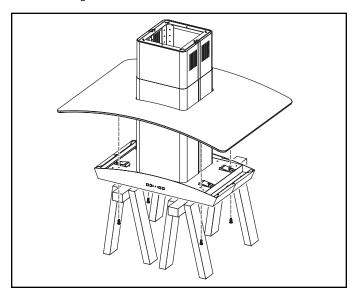
12. Place hood on a set of sawhorses. Carefully place glass canopy on top of the hood. To avoid damage to glass, make sure inside edge of glass cutout does not contact hood. Align nuts on glass canopy with holes inside the hood. Attach canopy with (4) .188" x .250" long flat head screws. Tighten screws securely but DO NOT OVERTIGHTEN.
