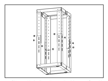
Disassemble the frame by removing (8) screws. Set aside screws and lower frame assembly.
