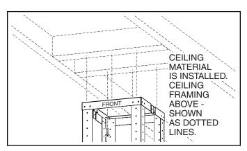
2. Align frame assembly to ceiling framing, and attach to ceiling framing with (6) 4mm x 50mm screws. Tighten securely, making sure that the upper frame bracket is tight against the ceiling.
