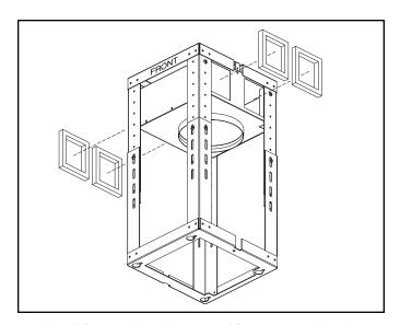
Attach foam seals to plenum and frame, around the plenum openings.
