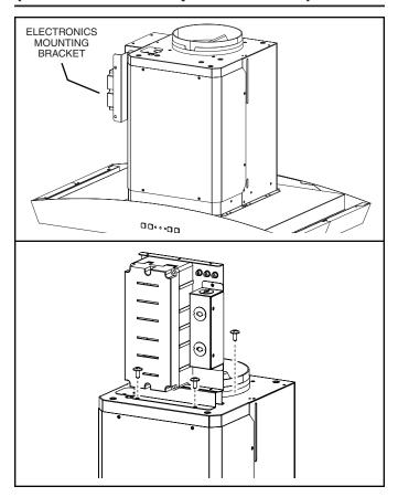
Remove tape holding electronics mounting bracket to hood. Remove (3) screws on top of hood chassis and set screws aside. Rotate electronics mounting bracket as shown and secure to hood with same (3) screws.
