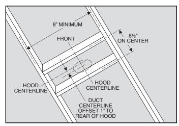
Construct wood framing that is flush with interior surface of the ceiling joists.
