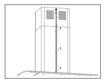
22. Carefully place the (2) lower flue sections on the hood frame, and overlapping the outside of the upper flue assembly, and nested into the glass cutout. Make sure that the clearance holes (larger) are in front of the attachment holes (smaller) where the two flue halves meet. While gently pushing the two flue sections together, attach the flue sections using (6) 3mm x 5mm screws.
