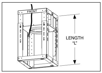
Determine length "L" of frame assembly based upon desired installation height. See chart on page 4. Slide lower frame over upper frame and attach with (8) screws previously set aside.
