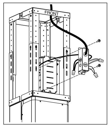
Remove wiring cover and connect house wiring to hood wiring – black to black, white to white, green to green. Reattach wiring cover.
