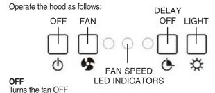
FAN (1-Pushbutton Switch, 3-Fan Speeds)
