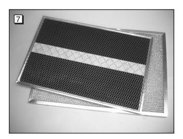
**To check filter:** Remove the filter clips and lift charcoal filter from grease filter to view indicator strip. Replace filter when the DOTTED LINES ON THE INDICATOR STRIP CHANGE TO WIDE SOLID LINES.
