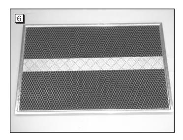
**Charcoal filters:** DO NOT immerse filters in water or put in dishwasher. The special "Clean Sense" feature indicates when filter is to be replaced. THE DOTTED LINES ON THE INDICATOR STRIP WILL CHANGE TO WIDE SOLID LINES. The "Clean Sense" feature works best when facing toward the cooking surface.
