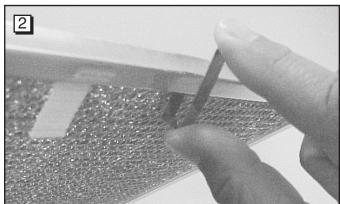
Place short end of clip against frame on "pull tab side" of aluminum mesh filter.
