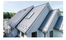
tion. Snap-Clad features an optional factory-applied sealant bead for improved weather resistance, a 1-¾-inch leg/seam height, and a continuous interlock for enhanced structural performance and wind resistance. The concealed-fastener clip system allows for thermal expansion and contraction while providing extraordinary hold-down strength.
