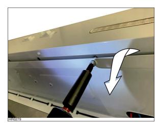
• Push the end of the BLUE wire through the electrical panel cover plate opening. Pull the RED and BLACK motor wires through the electrical panel cover plate opening.
