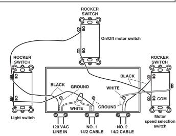
Install 3 rocker switches at a convenient place for the user. Feed the switch box with 120 VAC house wiring and use two 14/2 cable to wire it to the range hood (see diagram above).
