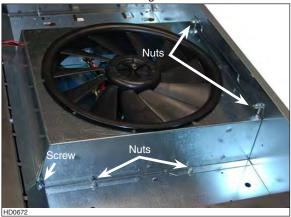
S Remove and set aside the 4 front screws retaining the bent plate to the hood.
