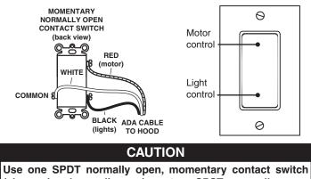
(shown in above diagram) or two SPST, normally open momentary contact switch.
