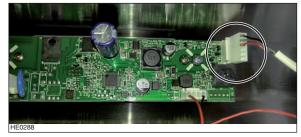
Secure the ADA cable section to the main harness using a tie-wrap.
