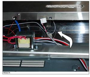
Onnect the ADA cable connector to the 6-pin connector on control board (circled on picture below).
