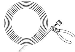
Run one end of the ADA cable through the range hood wire clamp, along with the power cable, giving enough lenght to make the connection inside the box. Tighten the wire clamp, then strip the end of the 3 wires from provided ADA cable.
