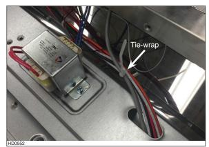
Olose the control access panel and reinstall the blower by reversing steps of to of on first page. Run the ADA cable section through the provided ferrite, making 2 loops. The ferrite must be as close as possible to the access panel.
