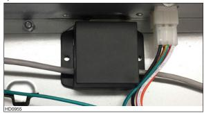
Reinstall the hood wiring cover and attach it to the hood using its retaining screw.
