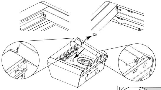
Using a 11/32" nutdriver or socket, remove the lock nut retaining the flange of the right blower cover plate (shaded part on illustration at right) to the inner back of hood (see inset). Remove all cover plate retaining screws (7 screws), then set the blower cover along with its screws and nut aside.
