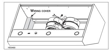
Rest the back cavity of the hood on wall extension metal tabs. Secure hood to wall extension using 8 provided no. 10-32 x 1/2" quadrex screws (4 on both sides). See illustration at right.
