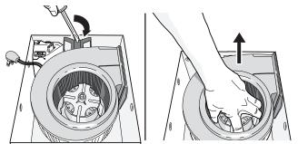
Remove wiring panel from fan housing. (if already installed).
