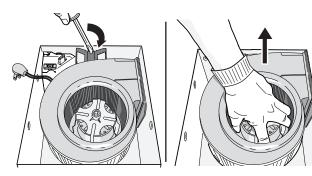
Remove wiring panel from fan housing (if already installed).
