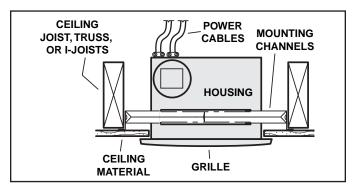
Housing mounted to joists, trusses, or I-joists. Up to 24-inches on-center.
