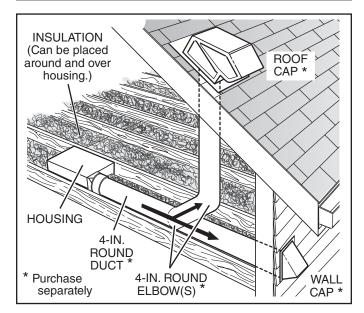
The unit will operate most quietly and efficiently when located where the shortest possible duct run and minimum number of elbows will be needed.
