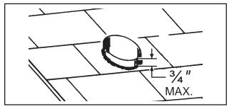
3. Trim ductwork parallel to roof pitch.
