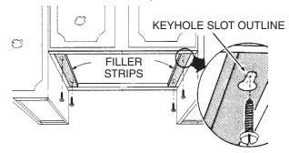
Screw the four supplied screws for mounting the hood into the exact center of the narrow end of the keyhole slots marked underneath the cabinet. Allow 3/8" of the screws to project, so the hood can be fitted into place.
