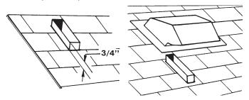
Roof Cap Discharge: Cut a hole in roof slightly larger than duct size being used. Trim shingles around hole so that they will fit snugly around hood of cap when cap is installed. Assemble the ductwork and tape all joints. Run ductwork down to hood location. Make sure that enough duct runs into the room so that the duct will overlap damper/duct connector when hood is put into place. Leave 3/4" of duct projecting above roof surface on high side.
