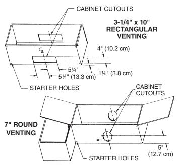
WARNING: WHEN CUTTING OR DRILLING INTO WALL OR CABINET, BE CAREFUL NOT TO CUT EXISTING ELECTRICAL WIRING.
