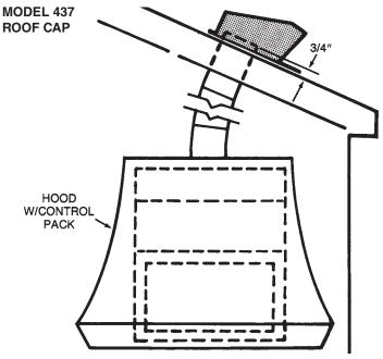
Cut a 10" round opening in the roof and extend the duct 3/4" above the roof on the high side. Nail roof cap down through flange on all sides (NOTE: If installed on a finished roof, insert upper edge of flange beneath shingles.) Use roof cement to seal shingles to top and sides of roof cap. Tape all duct connections.
