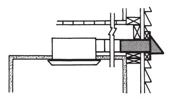
FRAME CONSTRUCTION: Use casing strips to space cap out flush with finished siding. Nail through flange on cap and into casing strips and sheathing. Connect fan to cap with 3" round duct. Tape all duct connections. Caulk around flange.
