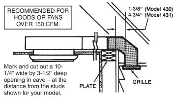
Insert discharge end of elbow (opening without the damper) over the top of the plate and down into the opening. Fasten discharge end of elbow to eave boards by nailing through the elbow. Connect the fan housing to the eave elbow with 3-1/4" by 10" duct. Fasten grille over eave end of elbow with the two wood screws provided.
