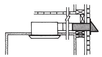
BRICK CONSTRUCTION: Position cap so that it will be flush with outer surface of brick. Nail in place through throat of cap. Connect fan to cap with 3" round duct. Tape all duct connections. Caulk around flange.
