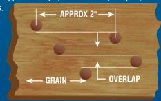
contain extensive holes where wood fibers are actually missing, it is recommended to mix sawdust with "GIT"-ROT® and use it as a fill material after treating area. In areas such as transoms, stringers, and balsa core decking, drilling thru the fiberglass surface may be necessary. For transom repairs, you may drill vertically down through the transom, and then pour in "GIT"-ROT®. For decking, drill thru the surface to treat the wood underneath.
