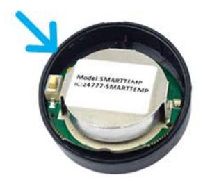
4. Align the button on the PCB with the button on the base of the sensor Press the base down until it is locked.
