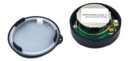
2. Carefully lift the board with the electronics. Replace the CR2477 battery.
