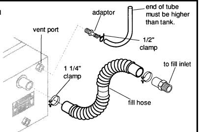
Screw adaptor into tank (supply port).
