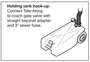
Emptying: Un-hook Tote-Along from coach. Pull to approved dump station. Vent Tote-Along by lossening 3/4" cap. Tip and dump.
