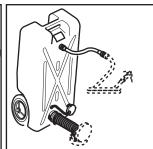
Cleaning: Attach hose to filler hose assembly and flush tank throughly.
