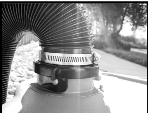
At campsite, take assembled sewer hose and attach one end on the top of the tank (as shown in this picture) and the other end to waste valve on trailer.
