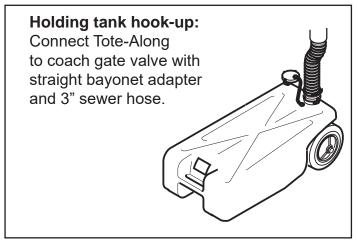
Emptying: Un-hook Tote-Along from coach. Pull to approved dump station. Vent Tote-Along by lossening 3/4" cap. Tip and dump.
