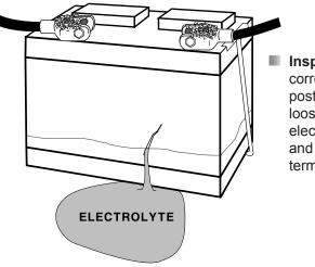
Inspect Battery for terminal corrosion, loose or broken posts, cracks in the case, loose hold-downs, low electrolyte level, moisture, and dirt around the terminals.
