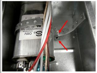
With the AC on a flat surface, remove outer shroud. Remove electrical box cover (2 screws).  Remove screw to loosen mounting strap securing the run capacitor. With vise grips, flatten strap surrounding existing screw location.
