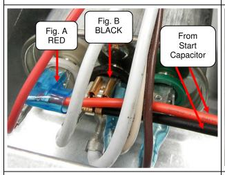
Connect wires from start capacitor to run capacitor. Connect RED wire to HERM terminal w/RED wire (Fig. A). Connect BLACK wire to COMMON terminal with WHITE wires (Fig. B).
